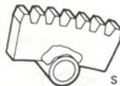
83 92 987 (A1) Locking segment for locking of crankshaft
