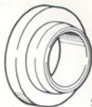
83 93 340 (A1) Sleeve, installation of seal on transmission side
