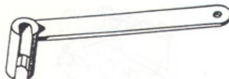
83 93 571 (A3) Spanner, removal and fitting of slave cylinder pressure line
